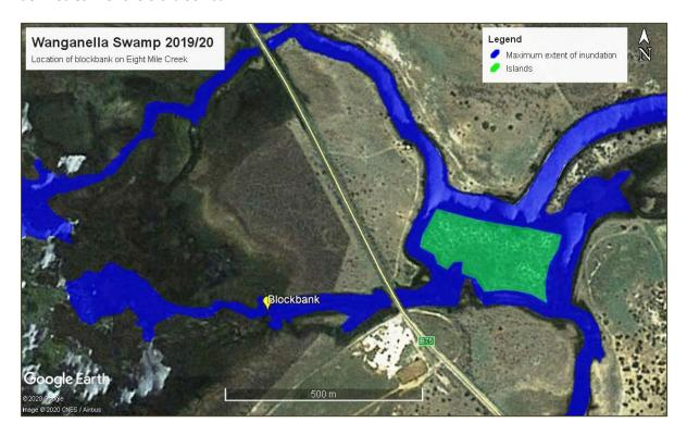
Figure 16: Location of the old block bank impeding flow via the southern Eight Mile Creek channel (Google Earth).
