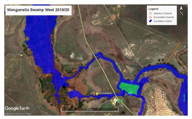
Figure 19: Map indicating the limited flooding east of the excavated channel marked with a red line (Google Earth).
